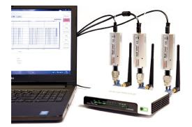
For MIMO devices with for example six antenna ports, an equal amount of RPR3006W power heads can be daisy-chained using the MMCX connectors enabling synchronised triggering of all six RadiPower meters. RadiMation Freeware captures the samples of each power meter simultaneously and calculates the total combined power according to the ETSI 300 328 standard.
